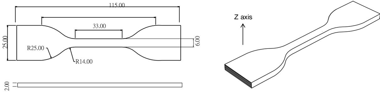
Tensile testing specimen; ISO 37
