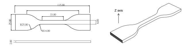
Tensile testing specimen; ISO 37
